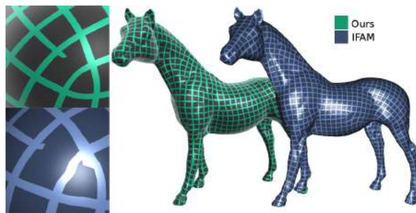
Fig. 17: Visualization of similar parameterization results of the same sphere model (left). The horse mesh (225k faces) parameterized with a cross-field by our method and the method by Jakob et al. [7] (right). Note that the cross-fields are not the same, since these are based on a random seeding.
