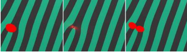
Fig. 8: Branch properties: Area around undefined phase (left), angular deviation of the parameter gradient and the vector field, where a full red location represents a deviation of 90^\circ (center), and angular deviation larger than 5^\circ (right).
