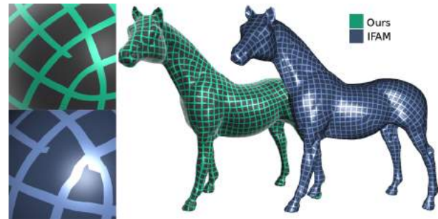
Fig. 17: Visualization of similar parameterization results of the same sphere model (left). The horse mesh (225k faces) parameterized with a cross-field by our method and the method by Jakob et al. [7] (right). Note that the cross-fields are not the same, since these are based on a random seeding.
